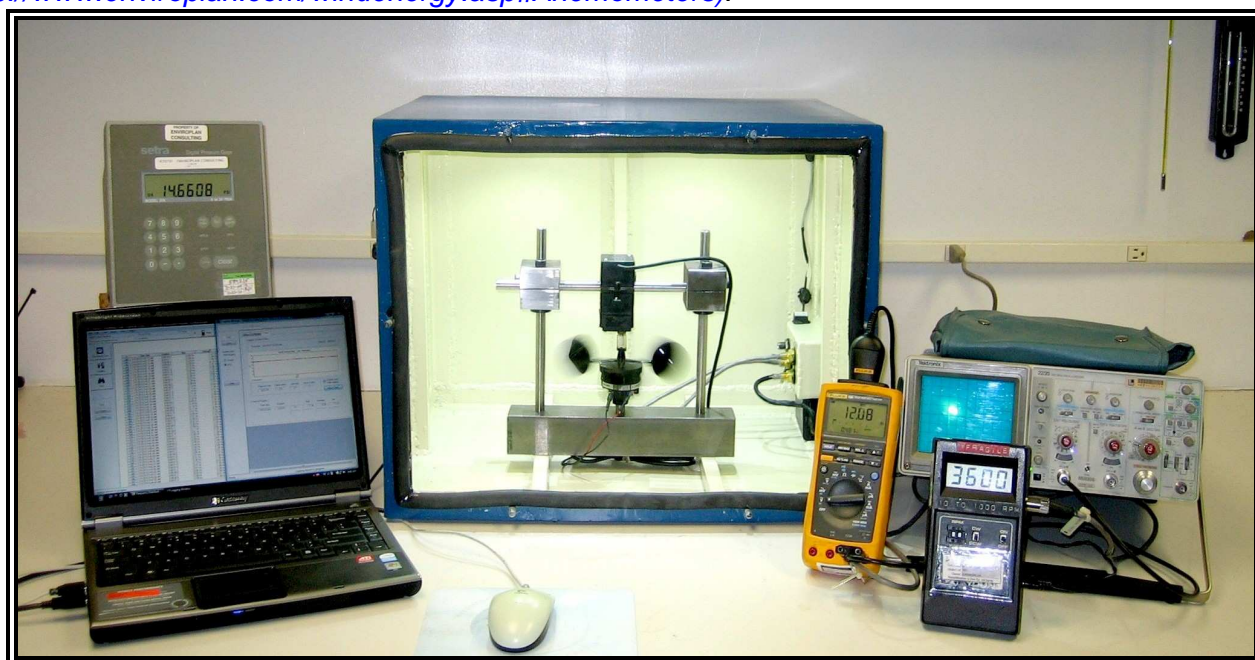
Calibration Test Apparatus for NRG #40 Anemometers
